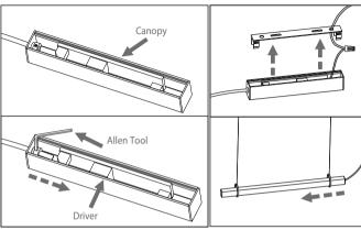
1º Fix the parabolt on the ceiling. Obs.: To fix on the concrete use the S4 Bushing and concrete screw (small). To fix in plaster/drywall use the Drywall Screw (big) with a specific bushing that is not contained in product package.
