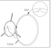
3º - Fix the cover on the lamp base, fixing first two of the rods, the third rod have to be align with the gap.
